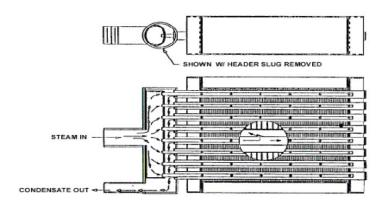
Steam distributing coils with a tow pass design have the same advantages of their multiple pass standard design counterparts. And like single pass steam distributing coils, these two pass coils work well in low or modulating steam applications and perform well when freezing air temperatures are encountered.
